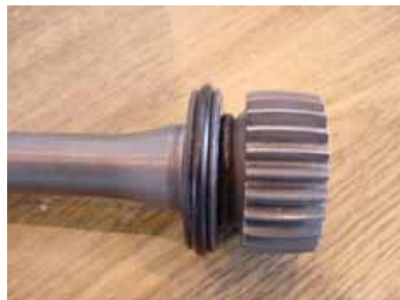
New shaft with seal & spacer
